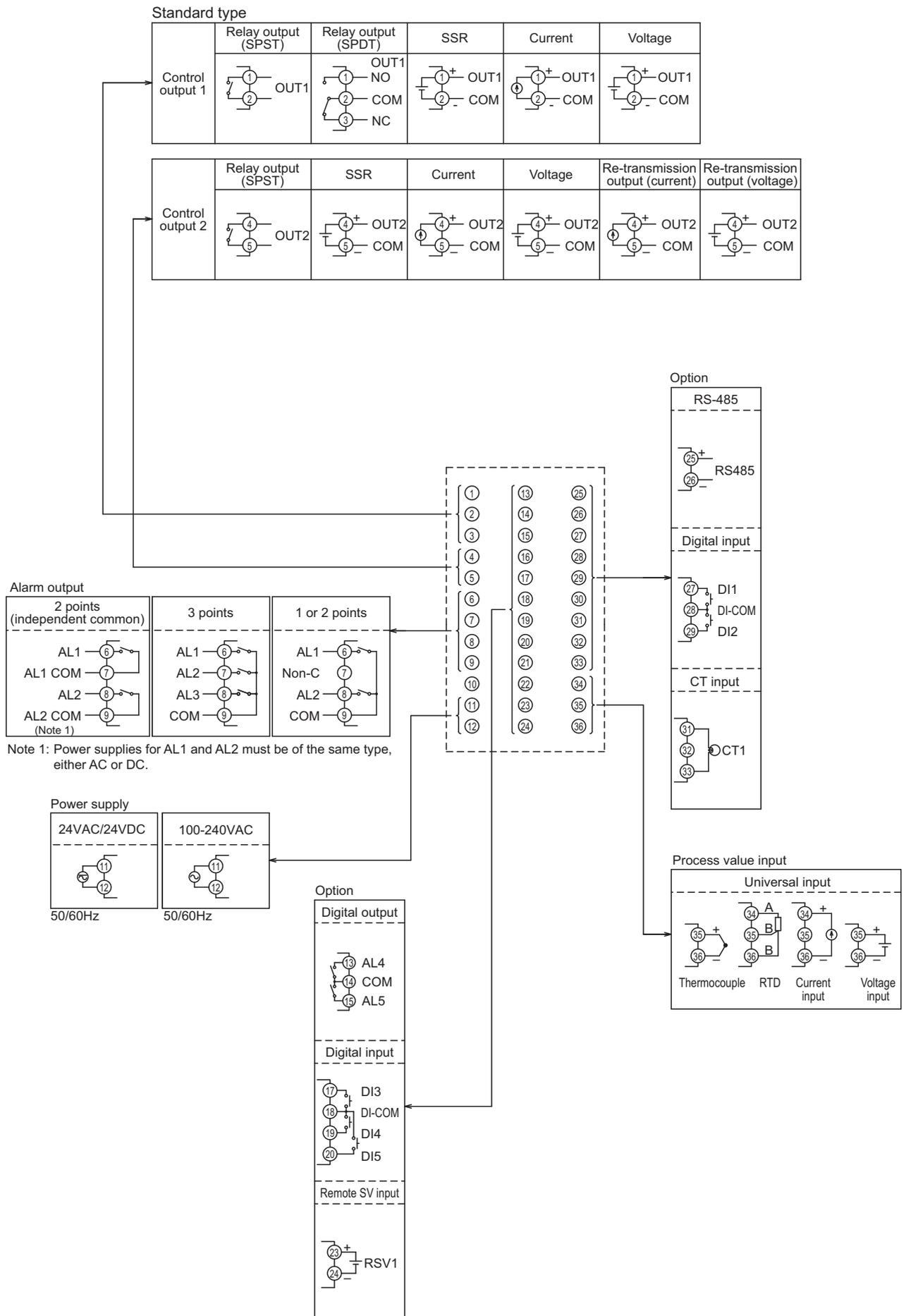
Motorized valve control type
