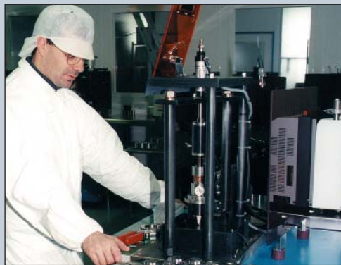
TIG welding : TIG (Tungsten Inert Gas) welding technology guarantees robust and reliable assemblies. These specialised welding facilities enable us to assemble the diaphragm seals, the capillaries and directly mount the seals on the transmitters. All welds are checked by a Helium tester to guarantee the integrity of the weld.
