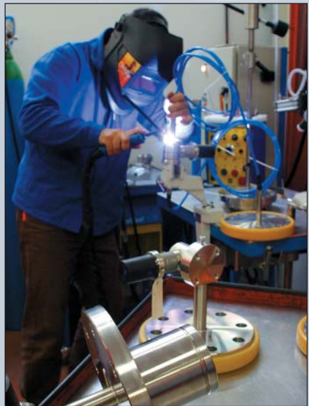
TIG welding : TIG (Tungsten Inert Gas) welding technology guarantees robust and reliable assemblies. These specialised welding facilities enable us to assemble the diaphragm seals, the capillaries and directly mount the seals on the transmitters. All welds are checked by a Helium tester to guarantee the integrity of the weld.
