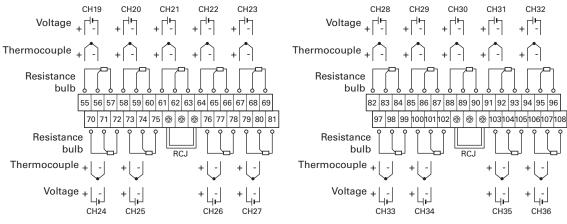
Note) For current input, connect an optional shunt resistance to a voltage input terminal.
