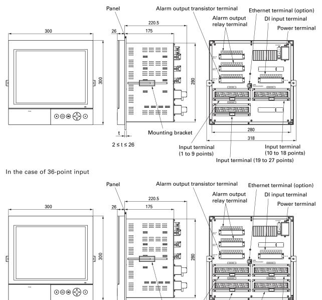
280 Mounting bracket t 318  $2 \le t \le 26$ Input terminal (1 to 9 points) Input terminal (28 to 36 points) Input terminal (19 to 27 points)
