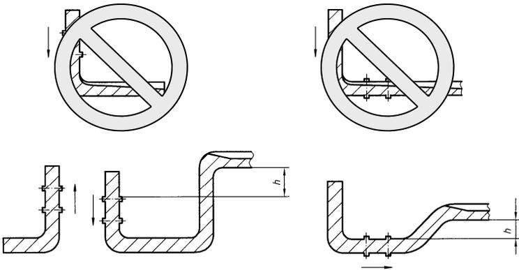
**Figure 2 - Proper Mounting Locations**
