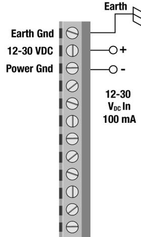
Figure 7 - DC Power Connections
