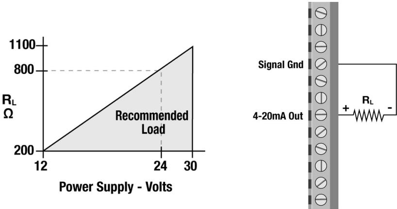
Figure 8 - 4-20mA Connections and Loop Resistance
