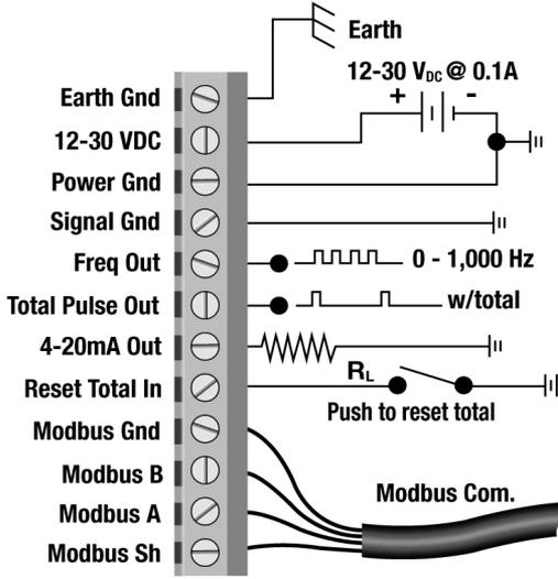
Figure 6 - FUSION Wiring Diagram
