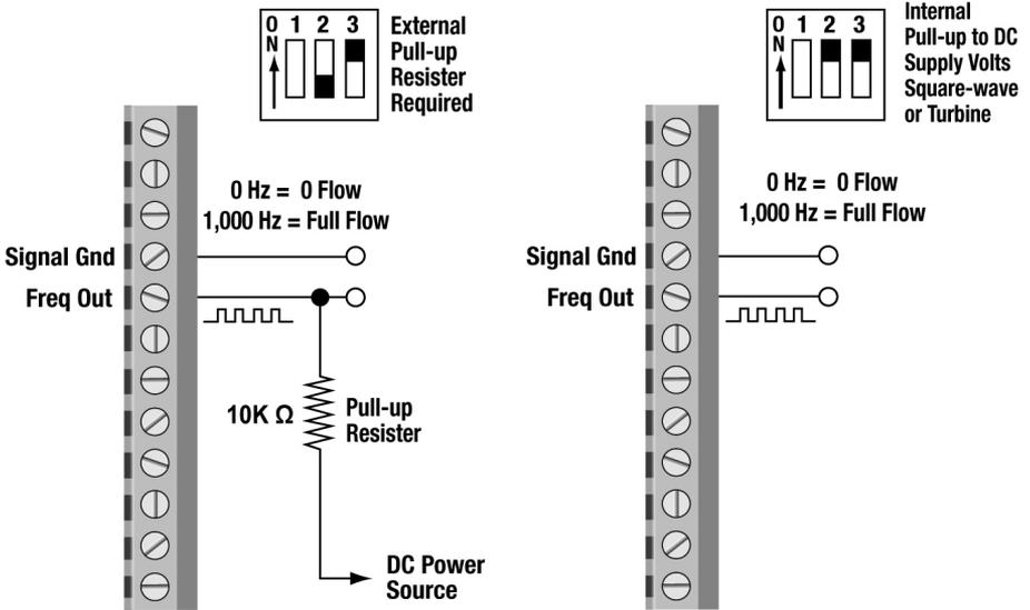
**Figure 10- Rate Pulse Output Connections**
