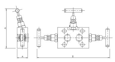
The 'Y34' and 'YV34' Type 3 valve manifolds are designed for direct mounting to differential pressure transmitters, with separate isolation for LP and HP inlets plus equalising valve for simple calibration. Each needle valve head is designed for safe and reliable isolation, giving bubble tight shut off, with non-rotating & antigalling tip and dynamic self-adjusting spindle seal to give long service life in a variety of service conditions.
