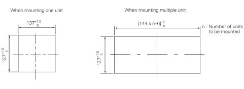
Note: When panel mounting, two bracket are necessary either on the top and bottom of the recorder.
