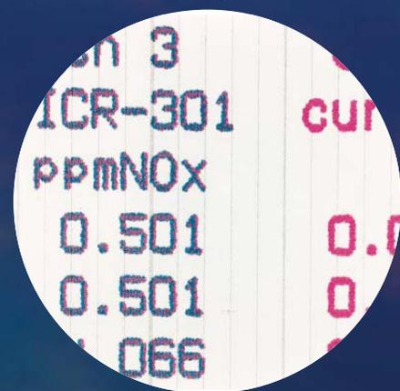
The ink jet printing mechanism allows continuous recording for a maximum of 12 channels (6 channels with 100mm width recorder) in 6 different colors. An A/D converter is used for each input signal for high speed data sampling to obtain a trace similar to that obtained by conventional pen mechanism recorders. Digital printing is also possible in the same color as the channel color, so clear and visible recording can be obtained.
