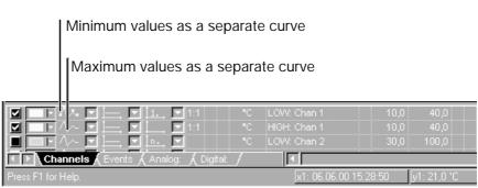
On screen recorders with an instrument software version that does **not** start with 100, two measurement curves are always available. The LOW curve includes the data for the acquisition types average value, momentary value, minimum value, maximum value, and the minimum value for peak value measurement. The HIGH curve only contains the maximum values for peak value measurement.
