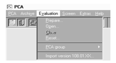
The *Evaluation* menu allows the graphical display of measurement values which are read out from the screen recorder, either via a diskette or via the communications server. The menu consists of the following functions:
