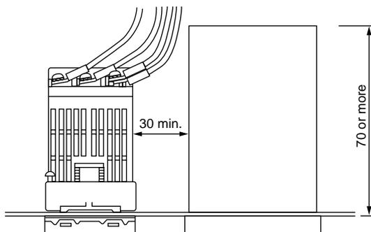
When there is another instrument (larger than 70mm) or a wall on the right side of this controller, be sure to install the controller keeping a space of more than 30mm.
