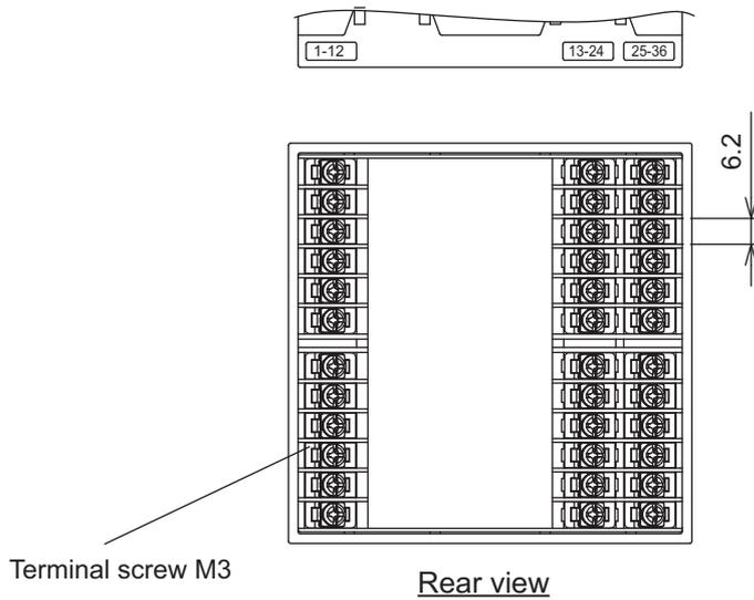
Terminal block is not attached to unused terminals (terminal 13 to 24) according to the model.
