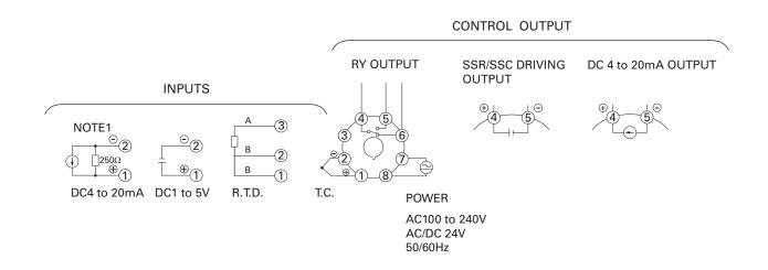
• <u>When compatible with PXW4/PXZ4/PXV4 resistance bulb input terminal</u> (When either one of the following is selected for the 5th digit of the code symbols: "N" and "S") Note that the terminal layout of the thermocouple input type differs from that of PXW4/PXZ4/PXV4.
