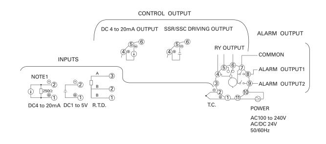
• When compatible with PXW4/PXZ4/PXV4 resistance bulb input terminal (When either one of the following is selected for the 5th digit of the code symbols: "N" and "S") Note that the terminal layout of the thermocouple input type differs from that of PXW4/PXZ4/PXV4.
