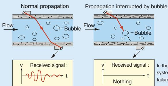
In the case of an analog system, measurement failure will occur.
