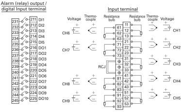
(Note) For current input, connect an optional shunt resistance to a voltage input terminal
