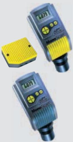
**MonoScan®** is an ultrasonic level measuring instrument for direct installation on tanks, vessels and reactors. It is a loop-powered 4-20mA device, with integral LCD display. Constructed of an ABS body, it features a sensor with a diameter of just 2" thread. **MonoScan®** is an excellent choice for measuring the level of liquids and solids at ranges of up to 15 meters (49ft), with a 0.25% accuracy of the measuring range.
