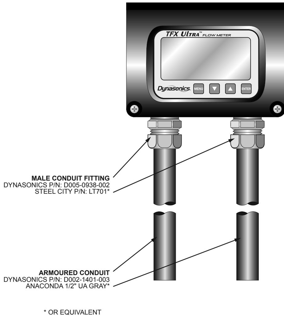
**FIGURE A-12.2 - CE COMPLIANCE DRAWING FOR DC POWERED METERS**
