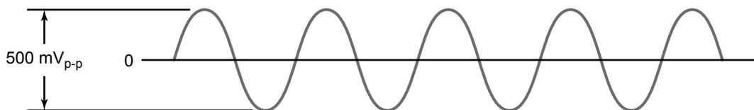
**FIGURE 3.7 - FREQUENCY OUTPUT WAVEFORM (SIMULATED TURBINE)**
