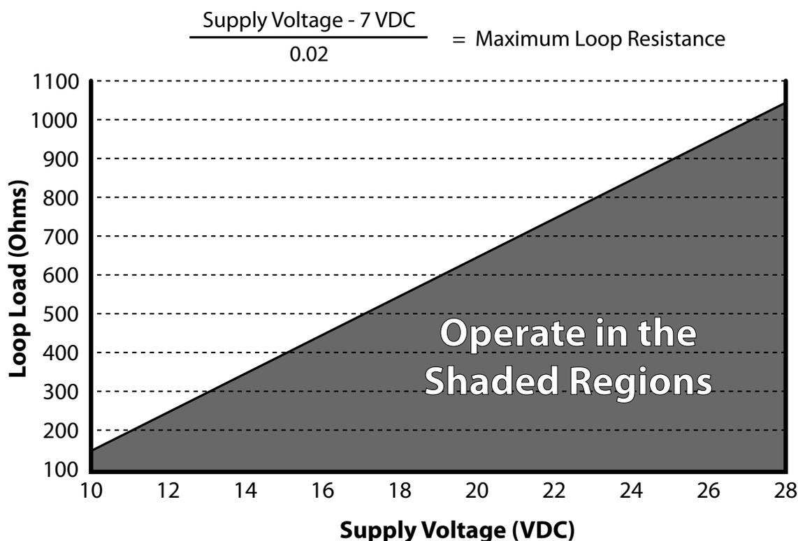
**FIGURE 3.1 - ALLOWABLE LOOP RESISTANCE (DC POWERED UNITS)**
