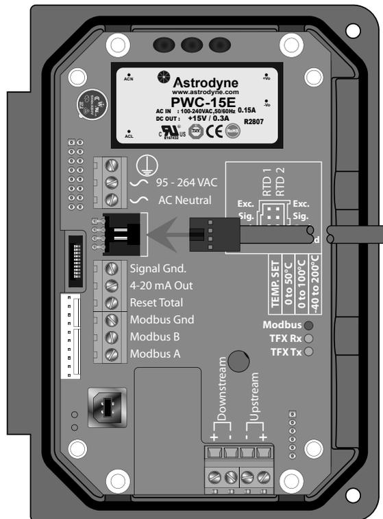
**NOTE:** Adding cable adds to the resistance the meter reads and may have an effect on absolute accuracy. If cable is added, ensure that the same length is added to both RTDs to minimize errors due to changes in cable resistance.
