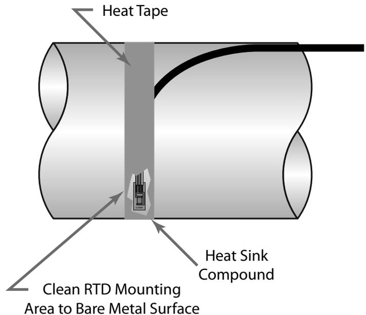
**FIGURE 3.11 - SURFACE MOUNT RTD INSTALLATION**
