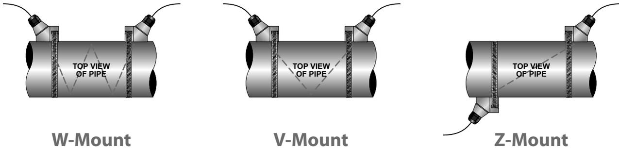
**FIGURE 2.1- TRANSDUCER MOUNTING MODES — DTTS, DTTL, AND DTTH**
