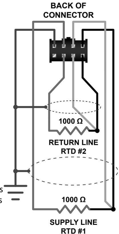
**FIGURE 3.10 - RTD SCHEMATIC**
