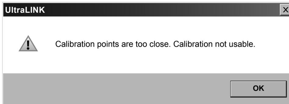
Check the RTDs resistance values with an ohmmeter to make sure they are not "open" or "shorted". See **Table A-4.2** for typical RTD resistance values. Next check to ensure that incorrect "Cal Point" values were not entered inadvertently.
