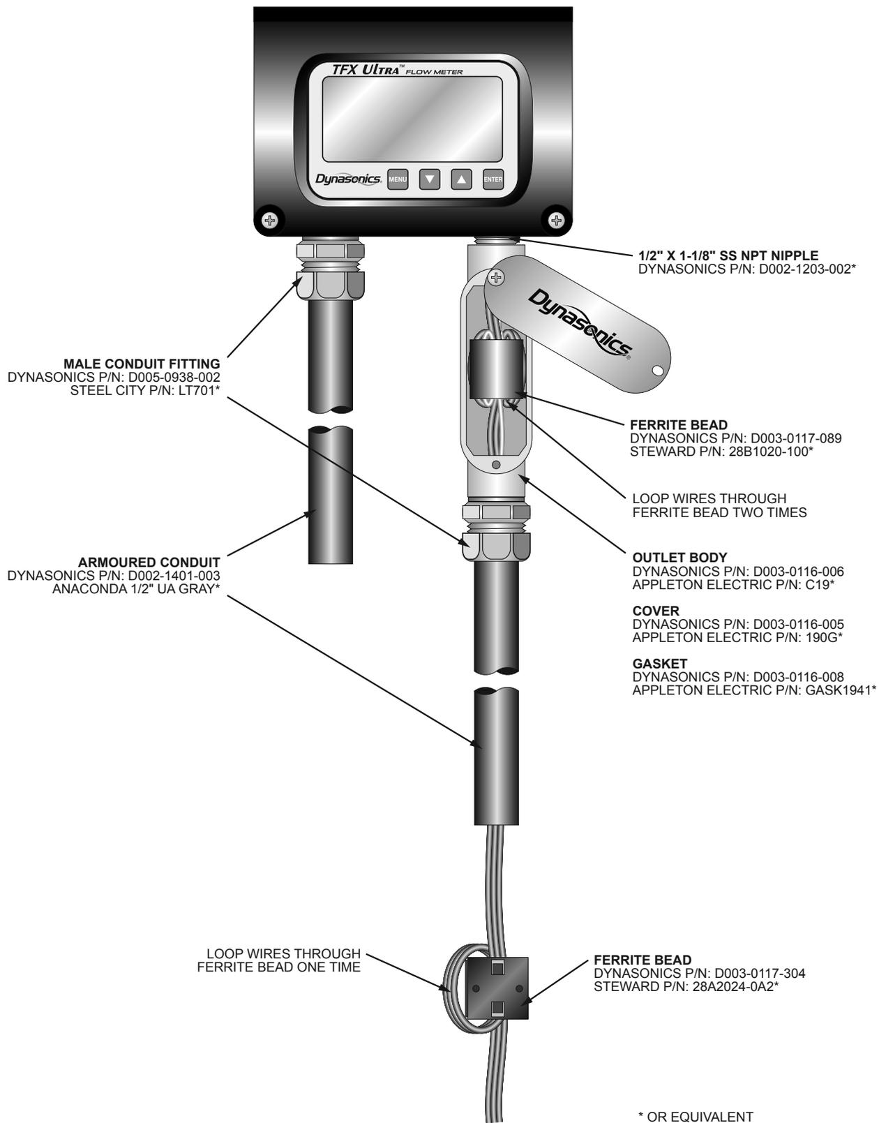
**FIGURE A-12.1 - CE COMPLIANCE DRAWING FOR AC POWERED METERS**
