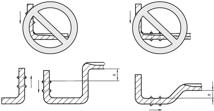
**Figure 2 - Proper Mounting Locations**
