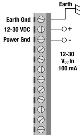
Figure 7 - DC Power Connections
