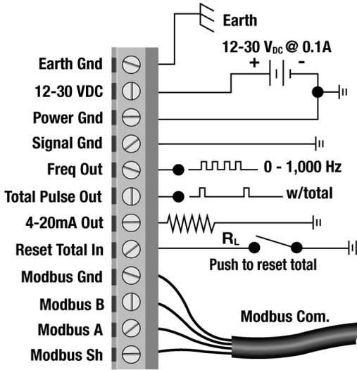
Figure 6 - FUSION Wiring Diagram
